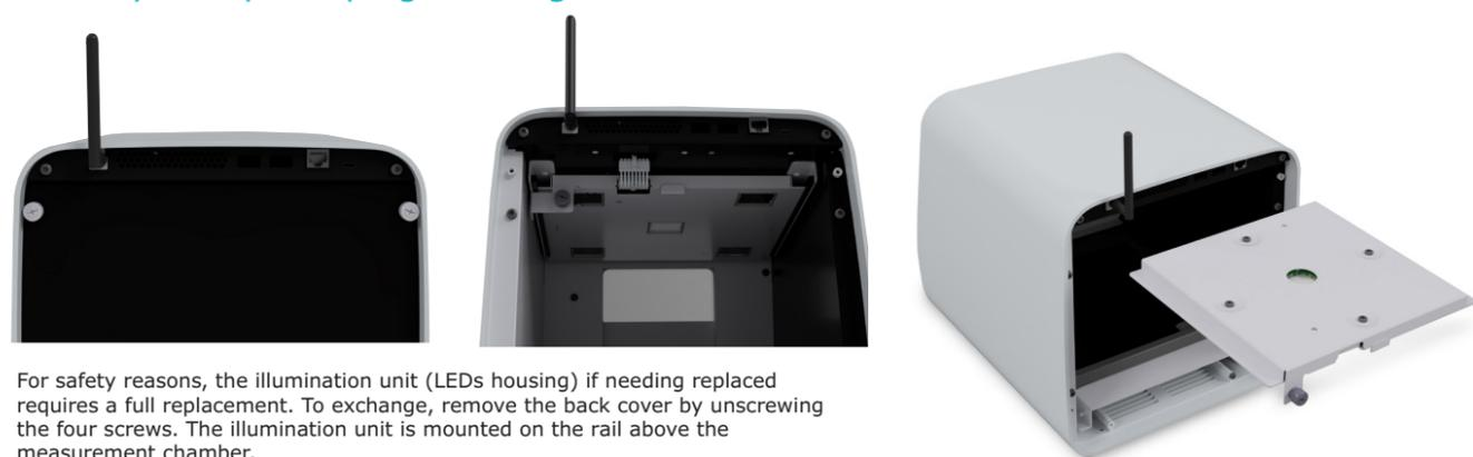
For safety reasons, the illumination unit (LEDs housing) if needing replaced requires a full replacement. To exchange, remove the back cover by unscrewing the four screws. The illumination unit is mounted on the rail above the measurement chamber.
