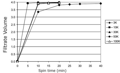
Spin conditions: 7,500  $\times$  g for 3K, 10K, 30K, and 50K, 5,000  $\times$  g for 100K, room temperature, 4 mL starting volume. Protein markers used: Cytochrome c for 3K and 10K, BSA for 30K and 50K, and IgG for 100K, n=6.
