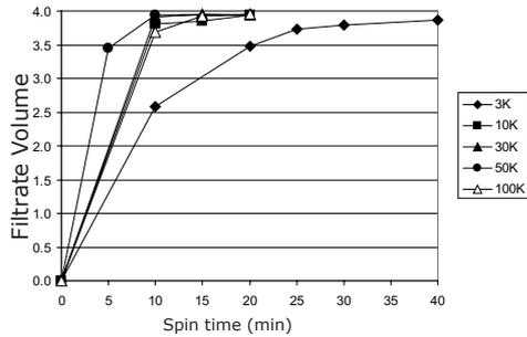
Spin conditions: 4,000  $\times$  g, room temperature, 4 mL starting volume. Protein markers used: Cytochrome c for 3K and 10K, BSA for 30K and 50K, and IgG for 100K, n=6.
