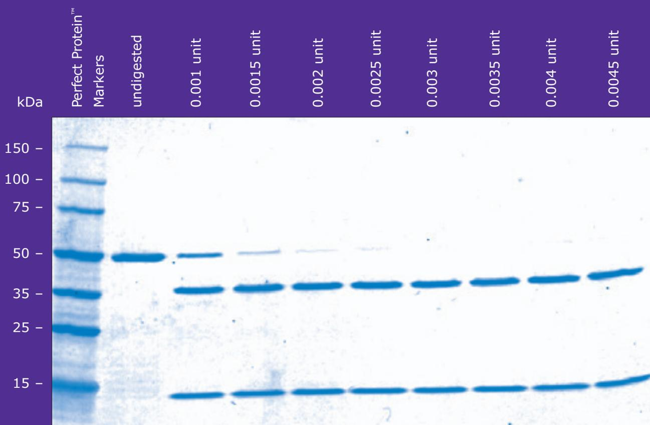
**Biotinylated Thrombin cleavage.** The indicated amounts of Biotinylated Thrombin were used to cleave 2  $\mu$ g of Cleavage Control Protein in an overnight digestion. Samples were analyzed by SDS-PAGE (4–20% gradient gel) followed by staining with Coomassie® blue stain. The 0.0045 unit lane represents a 2.25-fold over-digestion.
