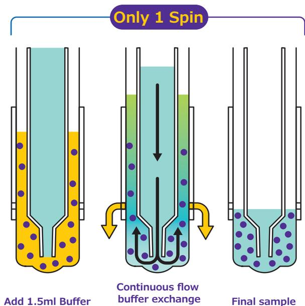
The uniquely designed interface between the exchange tube tip and the Amicon® Ultra device enables greater than 99% buffer exchange in a single spin. Buffer exchange, as shown in this diagram, was measured by the replacement of a low-molecular weight dye (yellow) with clear buffer (black arrows); while a high-molecular weight dye (bright blue) was retained inside the Amicon® Ultra device.
