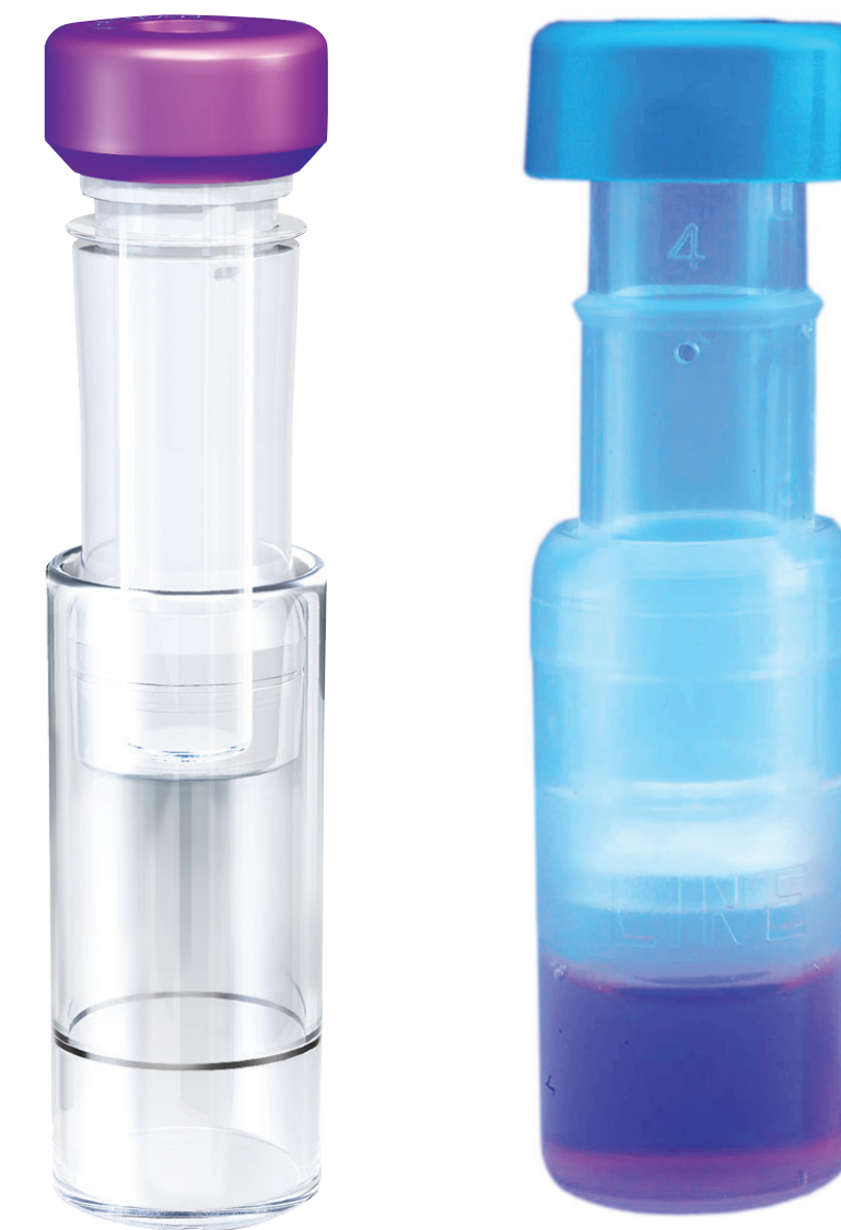
Fig 2: Mini-UniPrep glass (left) and plastic versions. Once compressed, the dimensions are equivalent in size to 12 mm × 32 mm vial.
