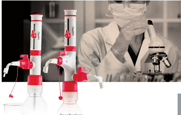
Accurate dispensing from an easy to use dispenser. LabPro Bottle Top Dispenser is a cost effective, safe, efficient, and durable bottletop dispenser, it has a re-circulation valve that re-directs liquid into the bottle to allow bubble free dispensing without any loss of reagent. Its smooth and soft plunger mechanism makes it easy to use in a demanding laboratory environment.
