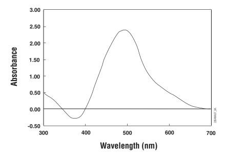
**Figure 3. Absorbance spectrum of MTS/formazan.** The absorbance spectrum of the formazan product resulting from reduction of the MTS tetrazolium compound shows an absorbance maximum at 490nm. The negative absorbance values (382nm) correspond to the disappearance of MTS as it is converted into formazan.
