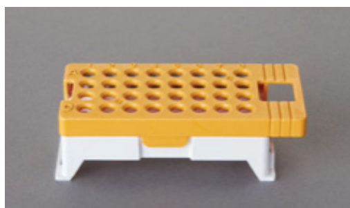
Figure 2. Assembled Spectrum Compact Sample Cartridge.
