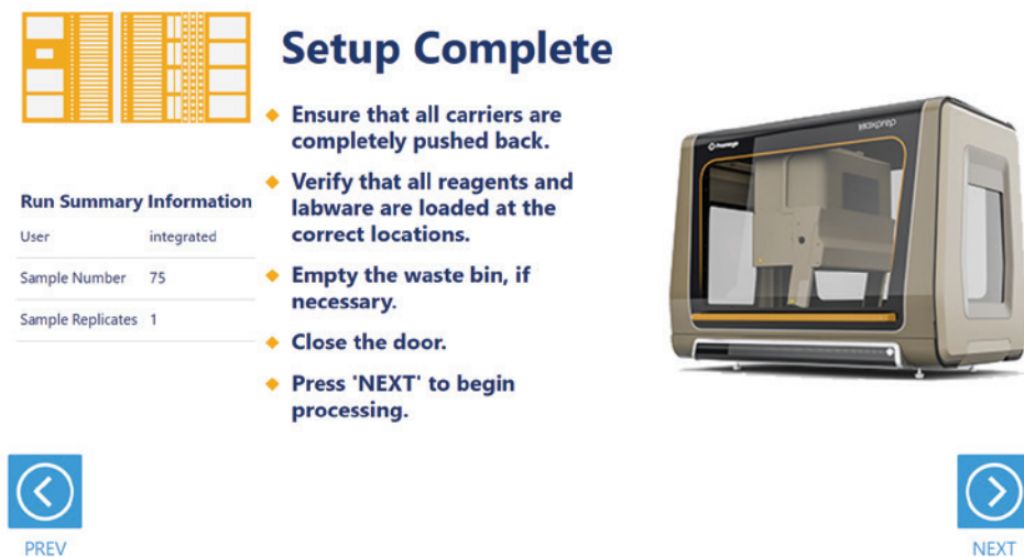
Figure 27. Final instrument setup screen. This screen presents a list of items that should be checked before starting automated processing. It also provides a final chance to return to any of the previous instrument setup screens before automated processing begins. To start processing, close the instrument door and press the Next button.
