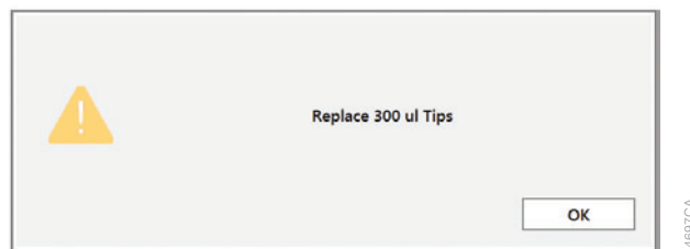
Figure 29. Insufficient tips on the system to complete a method. In the event that all tips of a given tip type are consumed during a run, the instrument will pause and unlock the door. Open the door, load more tips of the indicated type on the tip and plate carrier, close the door and press OK to resume processing.
