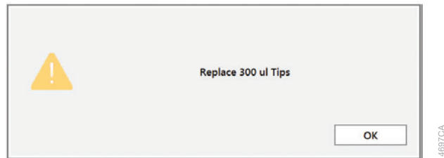
Figure 22. Insufficient tips on the system to complete a method. In the event that all tips of a given tip type are consumed during a run, the instrument will pause and unlock the door. Open the door, load more tips of the indicated type on the tip and plate carrier, close the door and press OK to resume processing.
