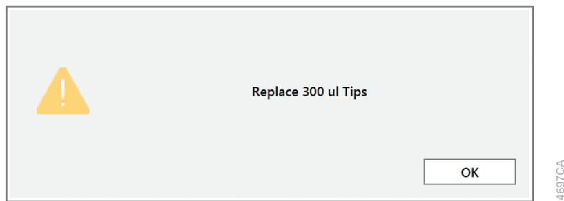
**Figure 18. Insufficient tips on the system to complete a method.** In the event that all tips of a given tip type are consumed during a run, the instrument will pause and unlock the door. Open the door, load more tips of the indicated type on the tip and plate carrier, close the door and press **OK** to resume processing.
