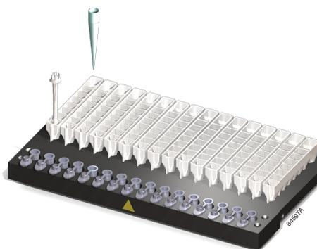
**Figure 3. Setup and configuration of the Maxwell® 16 LEV Cartridge Rack.** The LEV plunger is placed in well #8 of the cartridge (the well closest to the Elution Tube), and lysates are placed into well #1 of the cartridge.
