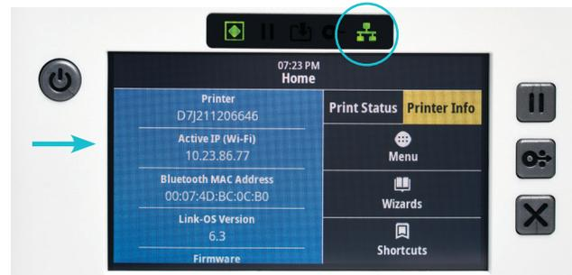
If the network connection is lost, the IP address will show only zeros and periods or the network indicator light will be red.
