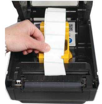
5. Gently pull the labels towards you, threading the labels underneath the Label Guides to secure them.
