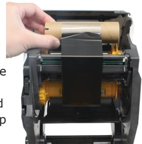
11. Take any slack out of the ribbon by gently turning the cardboard core adapter/take-up spindle away from you. The spindle will click as you roll it. Ribbon is now installed.
