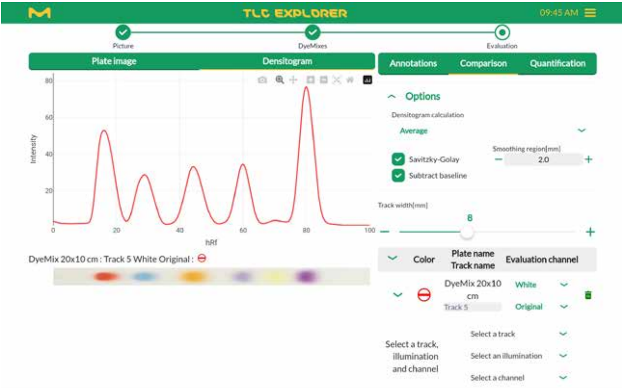
Figure 4.16: Edit densitogram calculation and display
