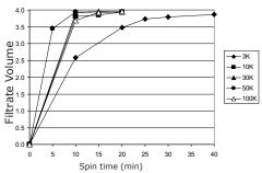
Spin conditions: 4,000  $\times$  g, room temperature, 4 mL starting volume. Protein markers used: Cytochrome c for 3K and 10K, BSA for 30K and 50K, and IgG for 10K, p.6
