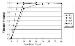
Spin conditions: 7,500  $\times$  g for 3K, 10K, 30K, and 50K, 5,000  $\times$  g for 100K, room temperature, 4 mL starting volume. Protein markers used: Cytochrome c for 3K and 10K, BSA for 30K and 50K, and IgG for 100K, n=6.
