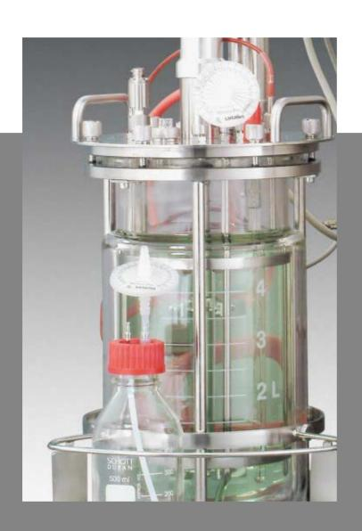
Midisart® 2000 The ready-to-use filter for sterilizing gases and venting
