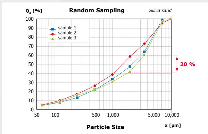
Therefore, it is essential that sampling is carried out with utmost care. A basic requirement for reproducible sieve analysis is the extraction of a **representative sub-sample** from the bulk. Representative means that the properties of the sub-sample, in this case the particle size distribution, have to be identical with those of the bulk.
