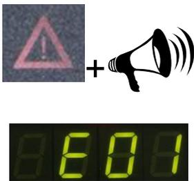
This safety feature functions independently of the control circuit. When the low-liquid-level protection device is triggered, the compressor and circulating pump are completely shut down and remain off.
