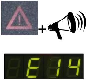
The high temperature cut-off is fixed at 85 °C and is independent of the control circuit. When triggered, the compressor and circulating pump are completely shut down and remain off. The alarm is indicated by optical and audible signals (continuous tone) and the "Error 14" message appears on the LED display.
