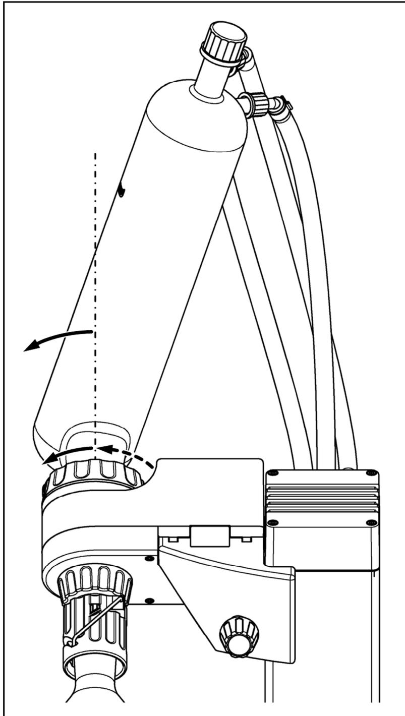
Fig. 4: Fully tightening the tension nut
