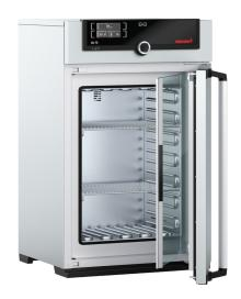
The heating of this incubator is optimally tuned for natural convection and valuable chamber loads for research, pharmaceutics, medicine and food chemistry are warmed up very carefully. On this page, you can find all the essential technical data on our incubator. Our customer relations team will be pleased to help if you want further information. If you should require a customised special solution, please contact our technical specialists at sales@memmert.com.
