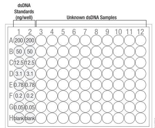
Figure 1. Dispense standard dilutions and blank samples in duplicate into Columns 1 and 2 of a multiwell plate.
