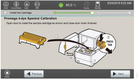
Figure 36. 'Install the Cartridge' screen.
