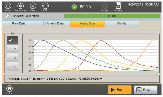
3. The 'Matrix Data' tab can be used to view emission spectra for each capillary (Figure 26).
