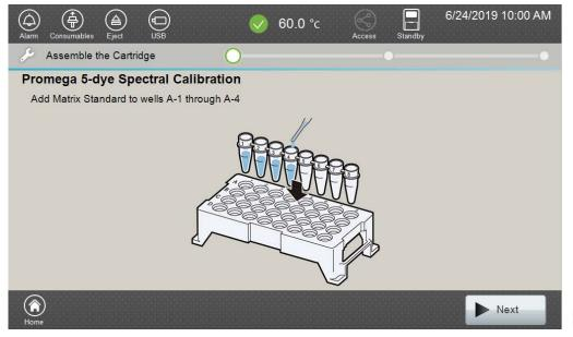
Figure 21. 'Assemble the Cartridge' screen.
