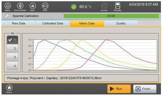
3. The 'Matrix Data' tab can be used to view emission spectra for each capillary (Figure 40).
