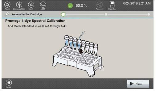
Figure 35. 'Assemble the Cartridge' screen.
