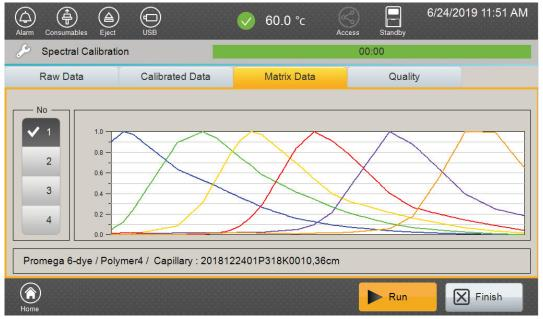
3. The 'Matrix Data' tab can be used to view emisson spectra for each capillary (Figure 12).
