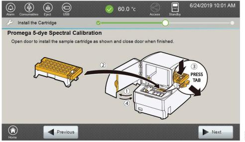
Figure 22. 'Install the Cartridge' screen.
