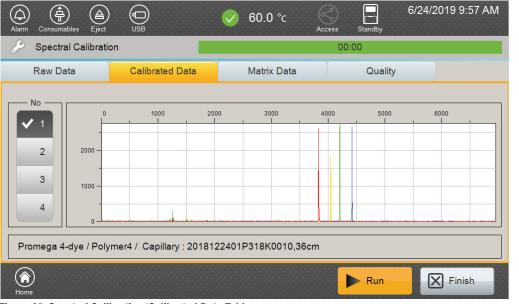
Figure 39. Spectral Calibration 'Calibrated Data Tab' screen.
