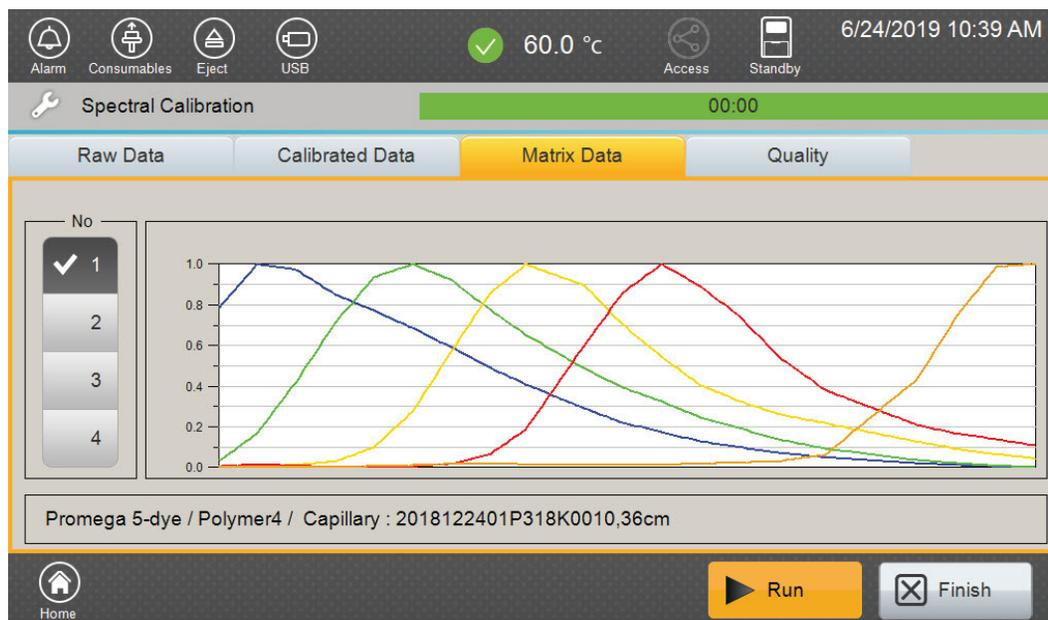
**Figure 26. Spectral Calibration 'Matrix Data Tab' screen.**
