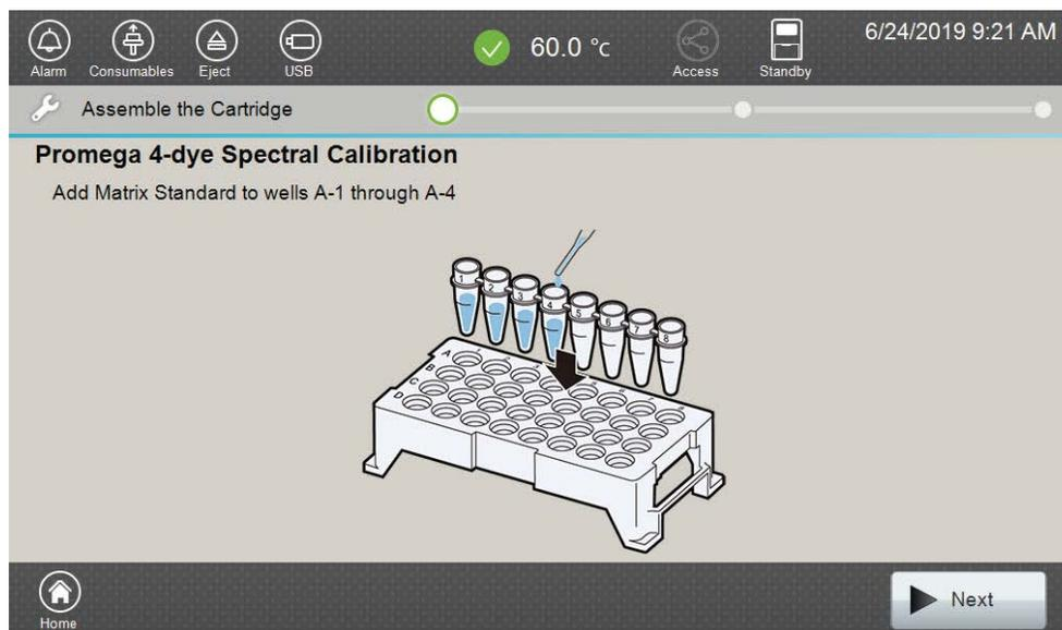
Figure 35. 'Assemble the Cartridge' screen.
