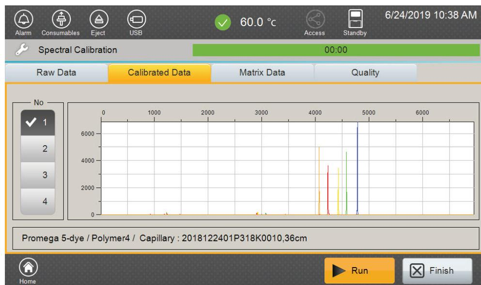
Figure 25. Spectral Calibration 'Calibrated Data Tab' screen.
