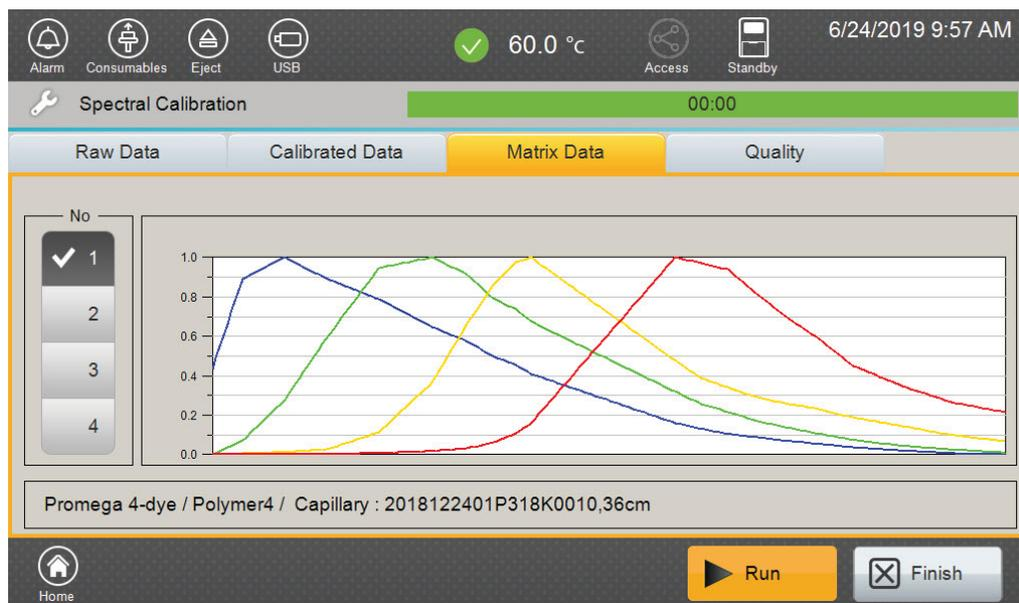
**Figure 40. Spectral Calibration 'Matrix Data Tab' screen.**
