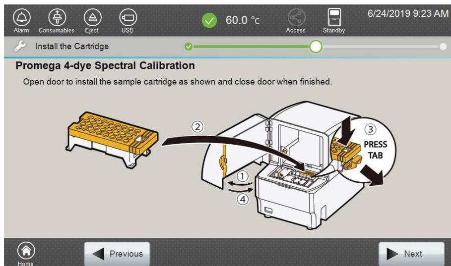
**Figure 36. 'Install the Cartridge' screen.**
