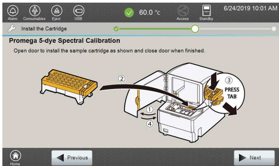
Figure 22. 'Install the Cartridge' screen.
