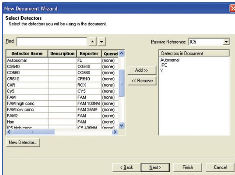
**Figure 24. Selecting the detectors and passive reference in the New Document Wizard window.**
