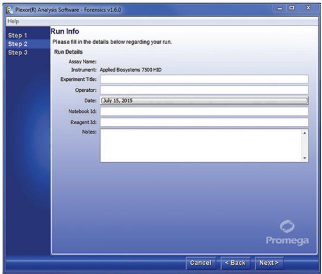
**Figure 19. Step 2 – Run Info screen. Enter run-specific information.**
