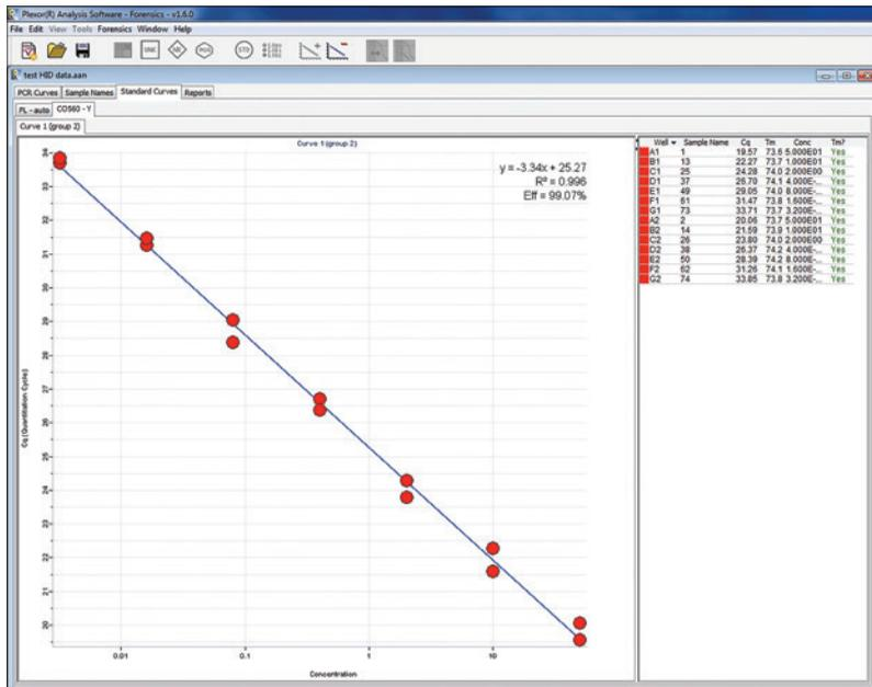
**Figure 39. The Standard Curves tab.**
