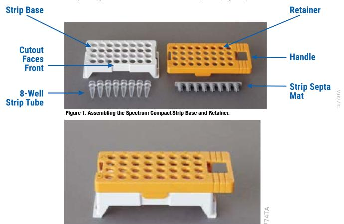
Figure 2. Assembled Spectrum Compact Sample Cartridge.
