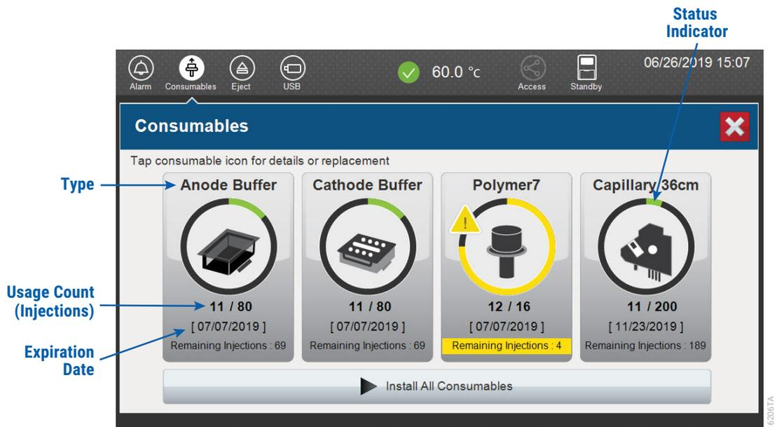
Figure 5. Spectrum Compact CE System 'Consumables' screen. Usage count (number of injections), on-instrument expiration date and remaining injections are displayed on the 'Consumables' screen for each consumable, as well as polymer type.
