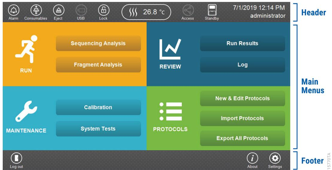
Figure 4. Spectrum Compact CE System Software 'Main Menu' screen.
