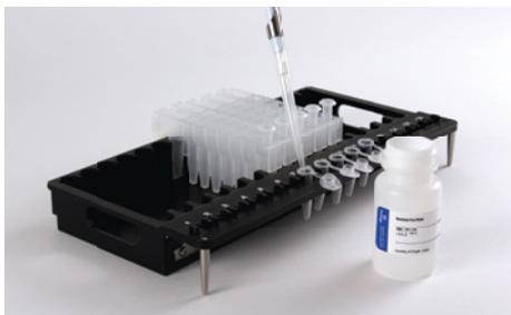
**Figure 2. Setup and configuration of the deck tray.** Elution Buffer is added to the elution tubes as shown. Plungers are in well #8 of the cartridge.
