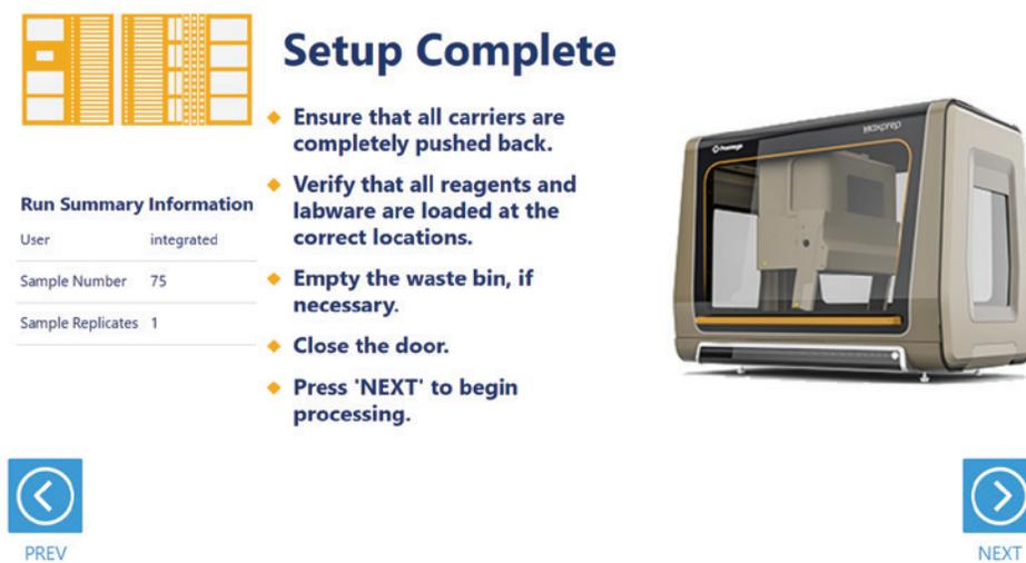
**Figure 21. Final instrument setup screen.** This screen presents a list of items that should be checked before starting automated processing. It also provides a final chance to return to any of the previous instrument setup screens before automated processing begins. To start processing, close the instrument door and press the **Next** button.
