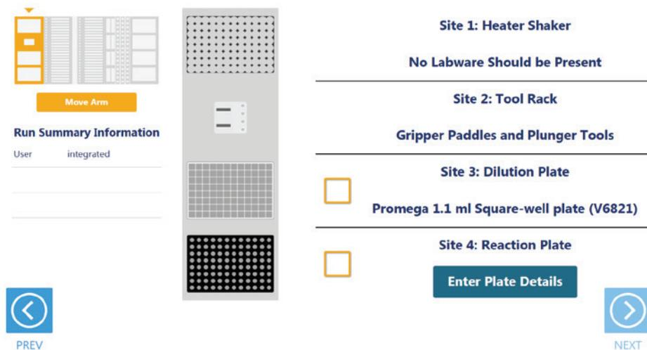
**Figure 12. Deck Setup screen for the Utility Carrier** This carrier cannot be removed from the system. It contains a Heater/Shaker for incubation of samples, tools and two labware positions. Place the indicated labware on the carrier, and check the boxes to activate the **Next** button. Press **Next** to continue instrument setup.
