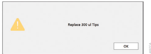
Figure 15. Insufficient tips on the system to complete a method. In the event that all tips of a given tip type are consumed during a run, the instrument will pause and unlock the door. Open the door, load more tips of the indicated type onto the tip and plate carrier, close the door and press OK to resume processing.
