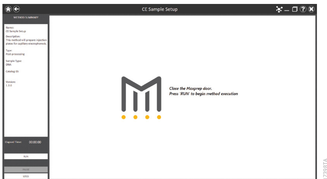
Figure 3. Method Run Environment screen. The Method Run Environment screen displays a summary of the selected method on the left side of the screen. Close the door of the instrument and select the Run button to begin method execution.
