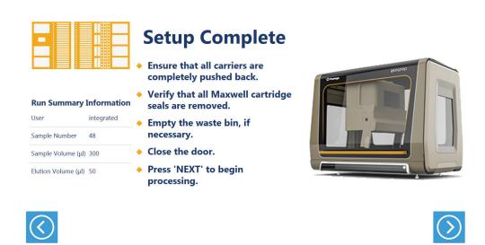
**Figure 15. Final instrument Setup screen.** This screen presents a list of items that should be checked before starting automated processing. The Final Instrument Setup screen also offers a final chance to return to any of the previous instrument setup screens before automated processing begins. To start processing, close the instrument door and select the **Next** button.
