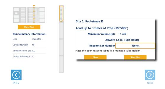
**Figure 10. Reagent Details information.** Details regarding the labware, minimum volume and reagent lot number can be accessed by pressing the **Enter Reagent Details** button for any occupied site on the reagent carrier.
