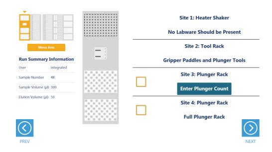
**Figure 5. Deck Setup screen for the first carrier.** This carrier cannot be removed from the system. The carrier contains a Heater/Shaker for incubation of samples, tools that the instrument will use for sample preprocessing and two labware positions.
