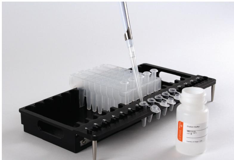
**Figure 1.** The CSC/RSC plunger is placed in well #8 of the cartridge (the well closest to the Elution Tube), and lysates and Lysis Buffer are placed into well #1 of the cartridge.
