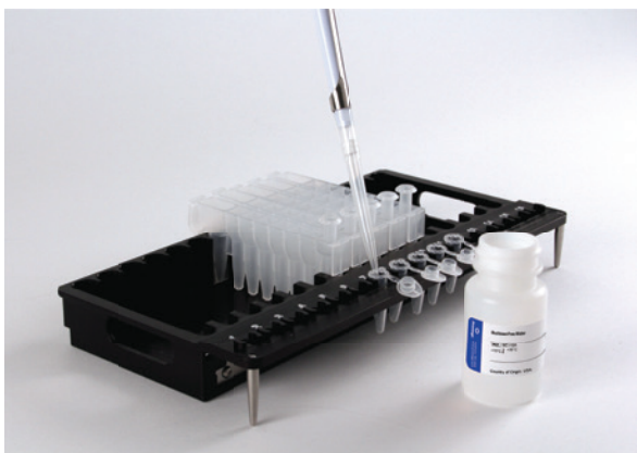
Figure 2. Setup and configuration of the deck trays. Nuclease-Free Water is added to the elution tubes as shown. Plungers are in well #8 of the cartridge.
