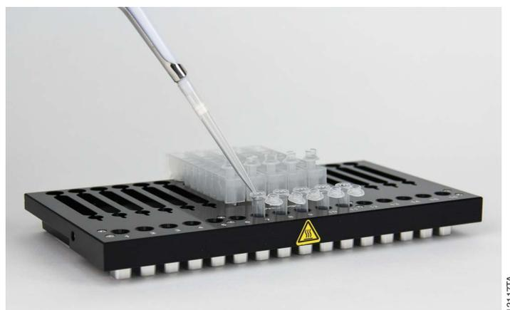
**Figure 3. Setup and configuration of the Maxwell® LEV Cartridge Rack.** Nuclease-Free Water is added to the Elution Tubes as indicated.
