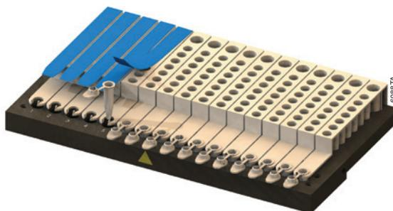
1. Place the number of cartridges to be used into the Maxwell® 16 LEV Cartridge Rack (Cat. # AS1251). Place each cartridge into the rack with the tube holder (Figure 1) facing towards the numbered side of the rack. Hold the cartridge firmly and remove the seal.
