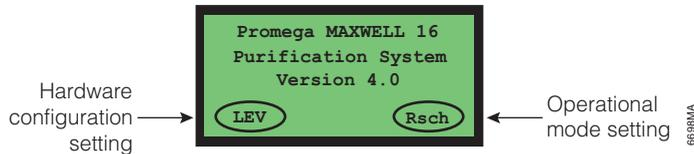
3. The current hardware configuration and operational mode settings are also displayed on this screen.
