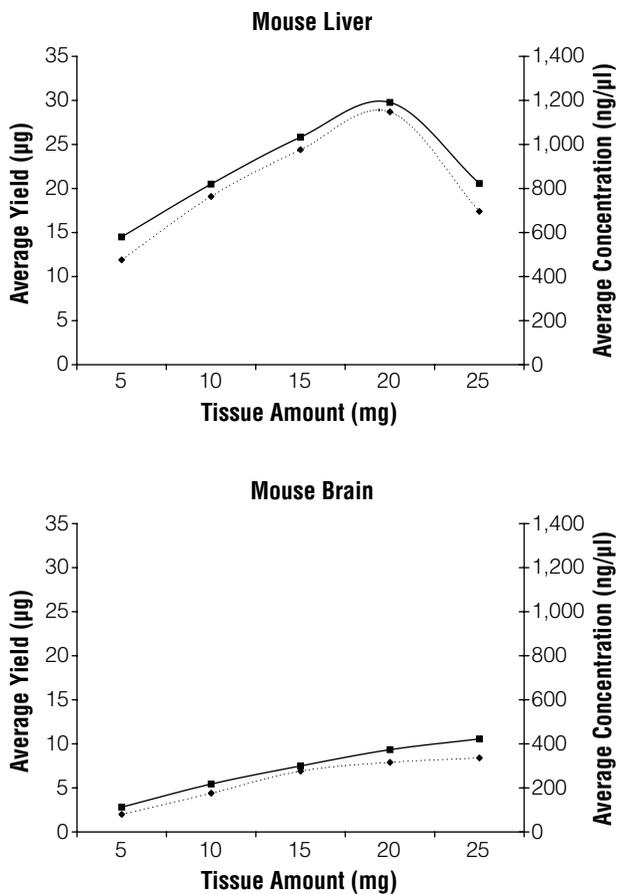
**Figure 3. Maxwell® 16 Tissue LEV Total RNA Purification Kit processing capacity will depend on sample type used.** Total RNA was purified from either 5, 10, 15, 20 or 25mg of mouse liver (a tissue with high RNA content) or mouse brain (a tissue with low RNA content) and eluted in 30µl of Nuclease-Free Water. The Average Yield (µg) of purified total RNA is plotted as a dotted line. The Average Concentration (ng/µl) of purified total RNA is plotted as a solid line.
