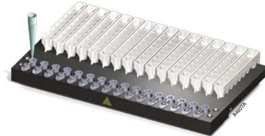
5. Place 0.5ml Elution Tubes into the elution tube holder at the front of the cartridge rack.
