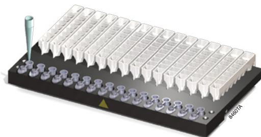
9. Transfer sample lysate to well #1 of the cartridge. Well #1 is the well closest to the cartridge label and furthest from the Elution Tube.
