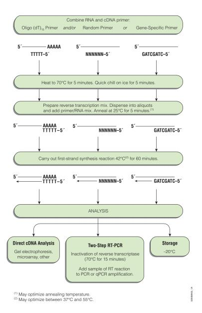
Figure 1. Schematic overview of cDNA synthesis and downstream analysis options using the ImProm-II™ Reverse Transcription System.
