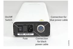
Figure 2. Rear view of the Power Supply showing the main power switch, fuse and power connections.
