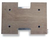
Figure 1. Place the instrument upside down on a stable surface. Remove the 4 screws holding the HSM 2.0 Instrument to the plywood.
