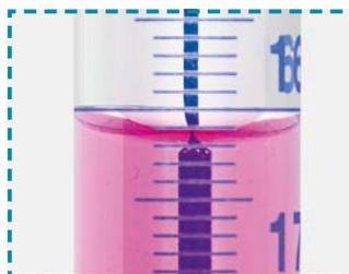
*The schellbach stripe has a narrow blue band which is at the center of the larger white band.*
